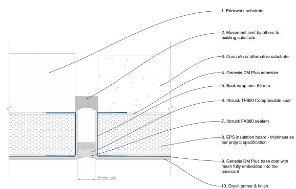
Movement joints should be installed generally @ 23 m max centres and to follow any movement /expansion joints in the existing substrate, at any transition /change to the substrate and at party wall locations
