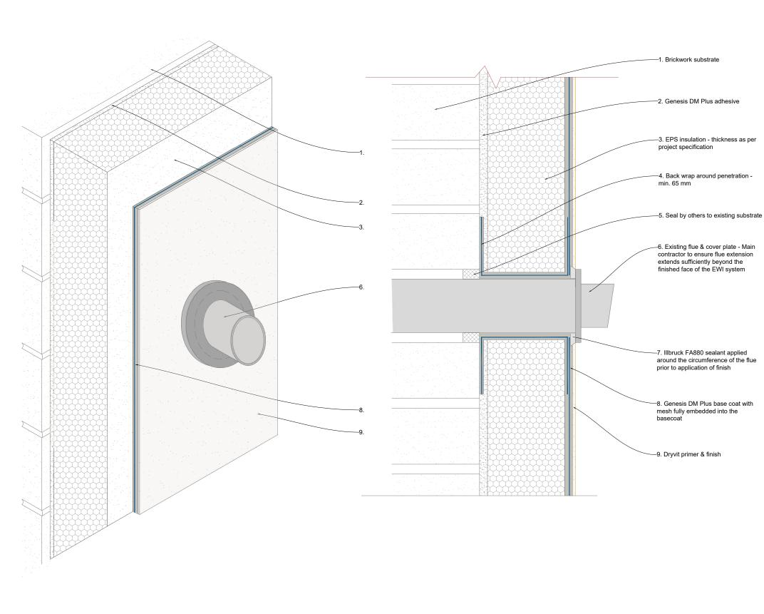
Note! The detail shown is suitable for a cold extract flue only. If there is any doubt whether the flue is hot or cold the detail for the hot extract flue must be used.
